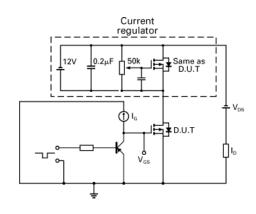
Basic gate charge waveform Gate charge test circuit
